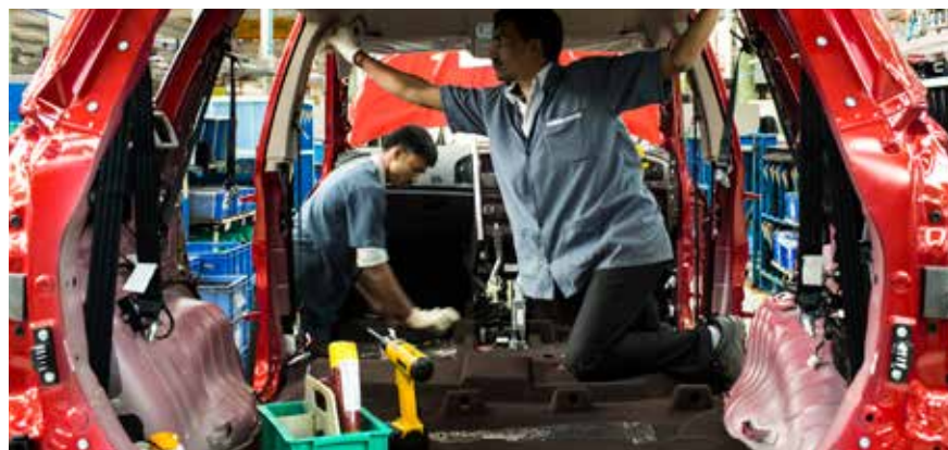
Employees install interior panels and fittings to a Mahindra & Mahindra Ltd. XUV 500 sport-utility vehicle (SUV) at the company's facility in Chakan, Maharashtra, India, on Sept. 12, 2014.
